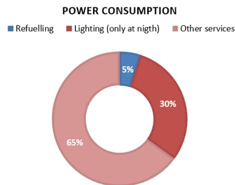
**Figure 4.3: Typical power consumption of a conventional retail station**
