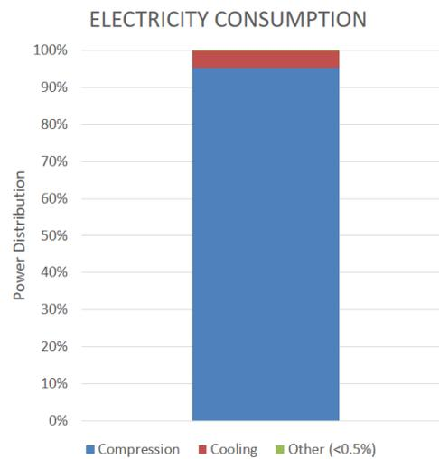
**Figure 4.2: Typical electricity consumption of hydrogen station (for an 80kg/day)**
