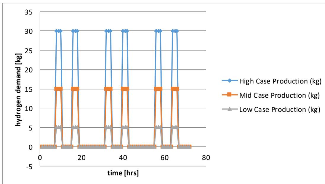
Figure 5.1: Hydrogen demand profiles for high, medium and low utilisation
