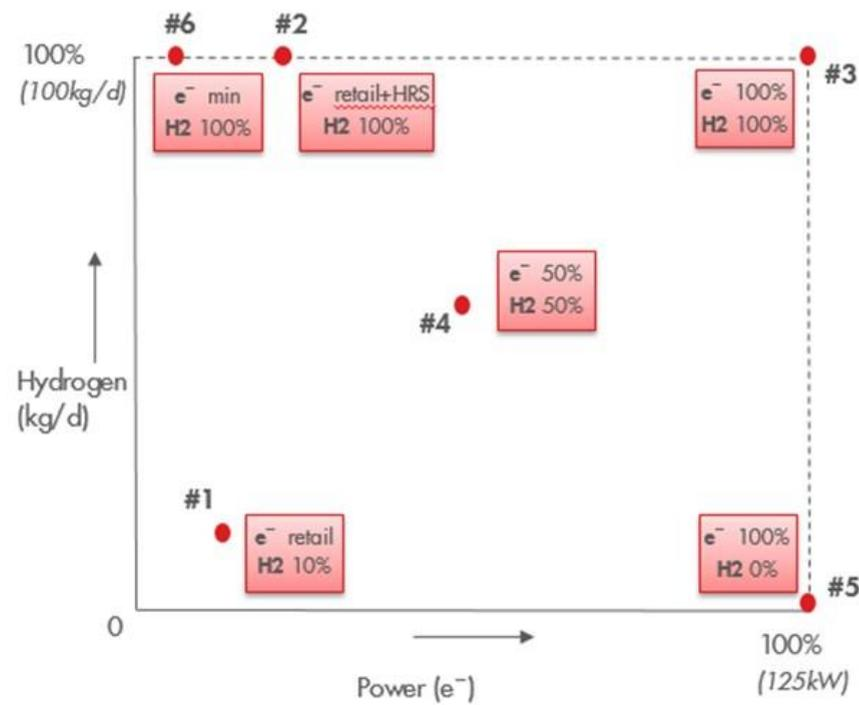
Figure 6.1: Operating envelope CH2P system
