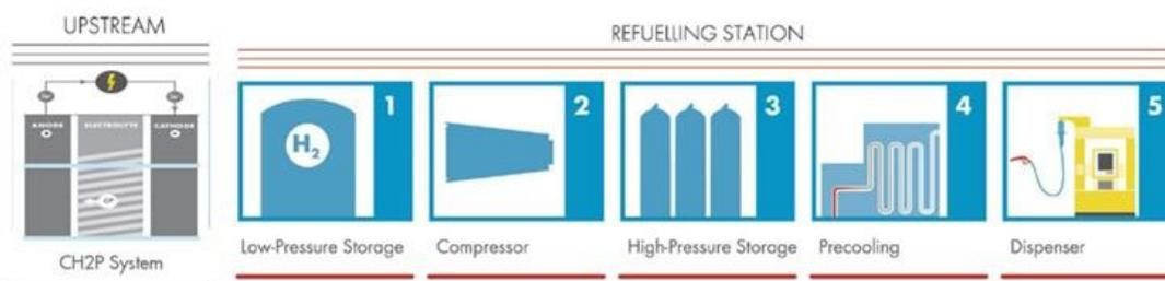
**Figure 4.1: Possible layout of a hydrogen fuelling station with CH2P system**
