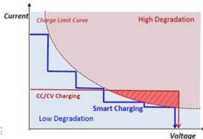
Figure 4.4: Example of a BEV smart charging curve
