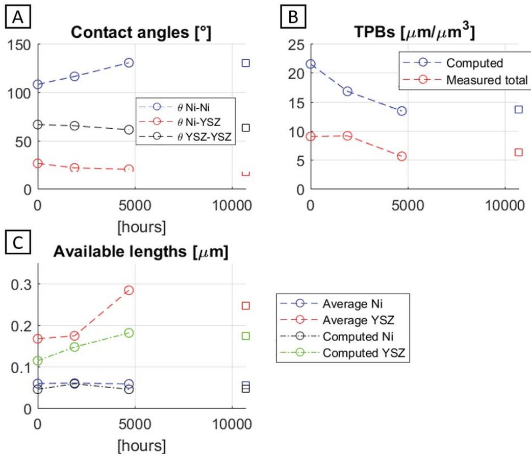
Figure 3: percolation theory-based model results. SOFC aged values are displayed with circle, SOEC aged ones with a square. (A) Contact angles between particles. (B) Total TPB lengths computed and measured (from Table 1). (C) Computed Ni and YSZ available lengths and computed averages (from Table 2).
