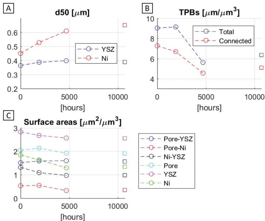
Figure 3: Evolution of measured topological properties (data referred to Table 1). SOFC aged values are displayed with circle, SOEC aged with a square. (A) Ni and YSZ d50. (B) Total and connected TPB lengths. (C) Interfacial and total surface areas.
